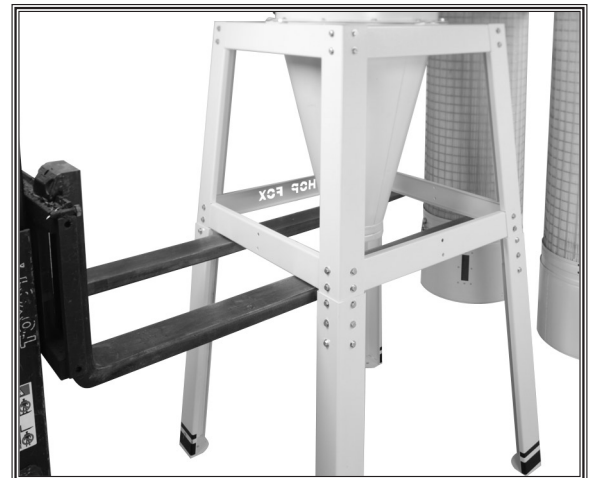
Figure 28. Lower stand legs attached (Model W1810).
